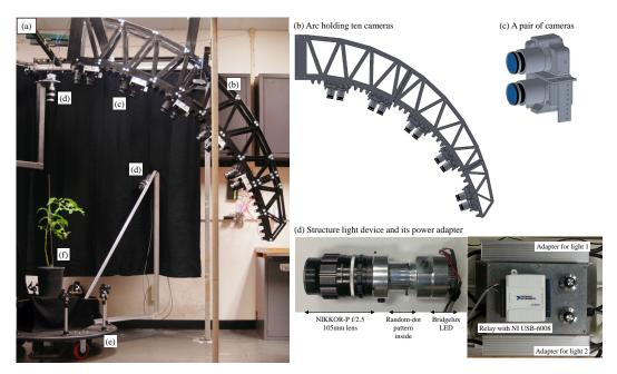
**Figure 1.** Mechanical structure (**a**) of the 3D reconstruction system: (**b**) the arc holding ten Canon EOS Rebel T3 cameras; (**c**) a pair of cameras where the second camera is upside down relative to the first one; (**d**) structured light devices and their power adapters with a relay controlled by a digital I/O control NI USB-6008; (**e**) a turn-table that rotates the plant 360 degrees; and (**f**) the target plant.
