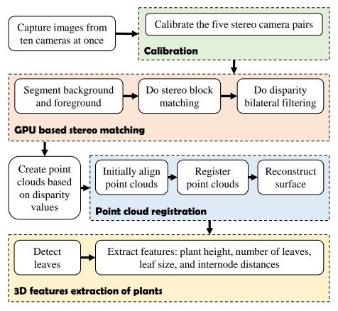
Figure 3. Block diagram representation of the software algorithm.
