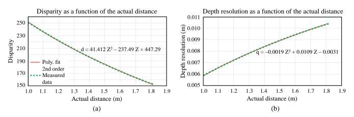
**Figure 6.** Estimation of the depth resolution of our stereo system as a function of the target distance from 1–1.82 m away from the camera: (**a**) Plot of disparities *versus* actual distances and (**b**) Plot of depth resolutions *versus* actual distances.
