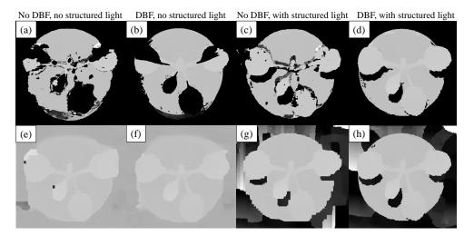
**Figure 5.** Results of the block matching (BM) (first row) and belief propagation (BP) (second row) algorithms with the use of disparity bilateral filtering (DBF) and structured light (SL): (a) BM result without SL; (b) BM + DBF result without SL; (c) BM result with SL; (d) BM + DBF result with SL; (e) BP result without structured light (SL); (f) BP + DBF result without SL; (g) BP result with SL; and (h) BP + DBF result with SL. The BM + DBF algorithm with SL is used in our system.
